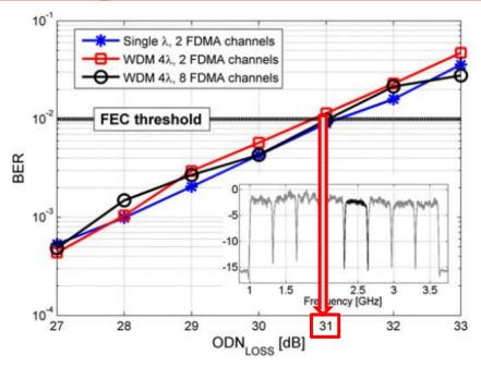
Fig. 2. Performance of the upstream transmission in terms of BER vs ODN loss with two active ONUs (32 emulated channels per wavelength using optical noise loading). It is evident that the simplified setup totally emulates the meaningful interferences.
