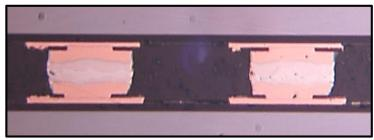
**20** μm Copper Pillar SnAgCu Solder Cap
