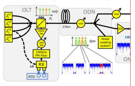
Fig. 1. Full off-line processing experimental setup with installed fiber, two active ONUs and r variable optical amplifier, RTO: real time oscilloscope, SOA: semiconductor optical amplifier, AB modulator, REAM: reflective electro absorption modulator).
