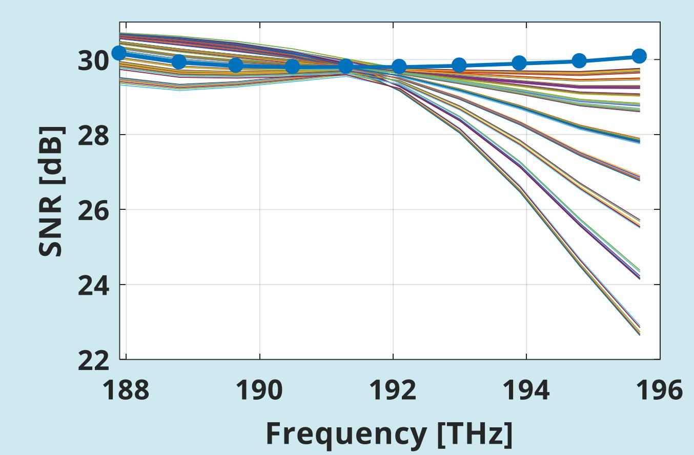
For optimal tilting we used GGN model to explore tilts between 0% and 200%. **50/0** (50% pre-compensation on L-band and 0% on C-band) is the tilt strategy which maximizes and flattens the SNR.
