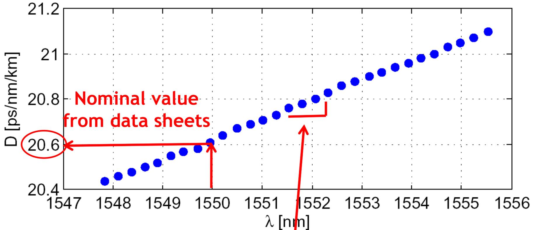
**Dispersion slope:  $0.057 \text{ ps/nm}^2/\text{km}$**
