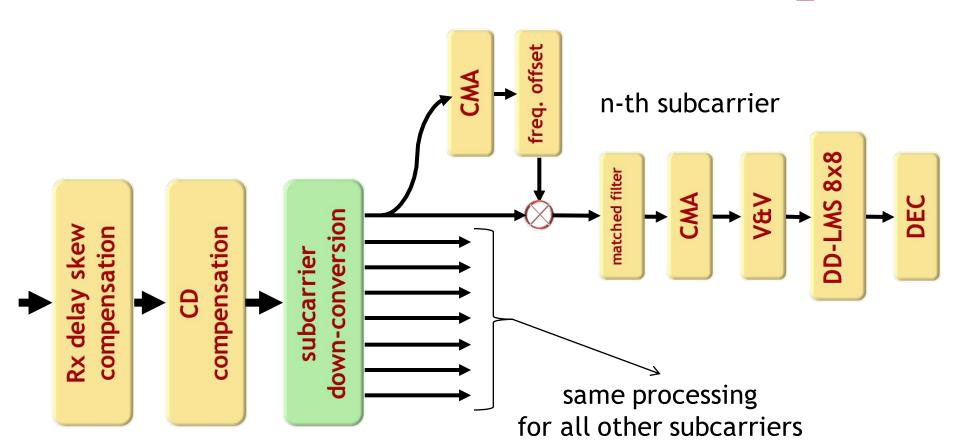
the 8x8 (real) LMS is necessary to correct for I/Q delay skew at the transmitter modulator (otherwise 4x4 is enough)
