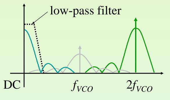
translated to base-band. In principle, due to beating with the other SCs, copies of this signal appears also around frequencies fVCO and 2·fVCO, but they are filtered out by the electrical receiver filter.
