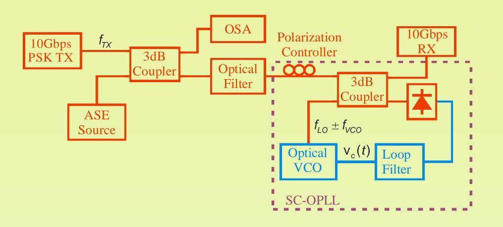
The Sub-Carrier OPLL (SC-OPLL) is our novel OPLL setup. It is the key element of the proposed coherent system.
