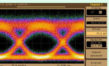
10Gbps IM-DD System OSNR=18 dB Measured Q = 15.8 dB
