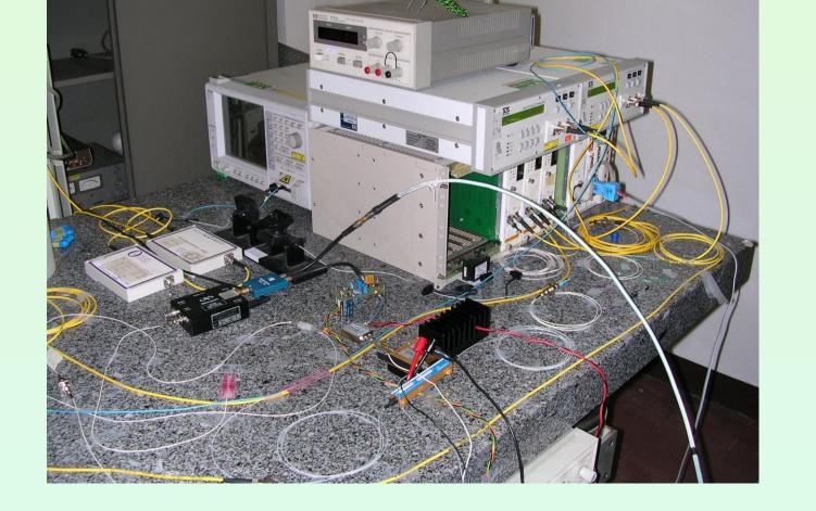
The transmitter is based on a Corning-OTI LiNbO<sub>3</sub> 10Gbit/s phase modulator, driven by an NRZ signal. The modulation voltage has been set to a slightly lower value than the modulator  $V_{\pi}$  voltage. The SC-OPLL locks the residual carrier.
