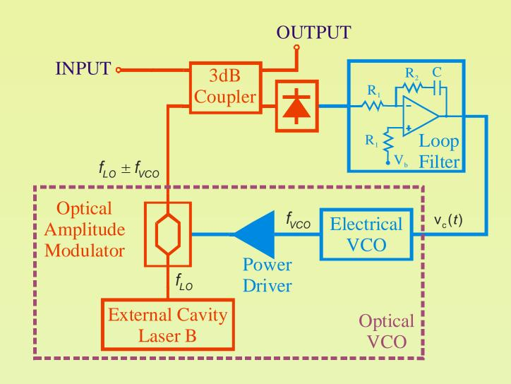
Two main Sub Carriers at frequency  $f_{LO} \pm f_{VCO}$  are generated. We are able to tune *both* by simply changing the voltage applied to the *electrical* VCO, thus implementing an Optical VCO.  $f_{LO}$  is set in order to obtain  $f_{LO}$ - $f_{VCO}$  equal to the received signal frequency  $f_{TX}$ .
