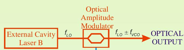
The amplitude modulator is a high bandwidth Corning-OTI LiNbO3 Mach-Zehnder (MZ) and is biased at a null of its transfer function,
