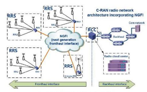
Figure 2-1: C-RAN Radio Network Architecture Based on NGFI
