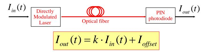
In DSP-aggregated fronthauling, many LTE radio waveforms are <u>frequency-division multiplexed</u> in the electrical domain, and then sent on an "analog optical link"
