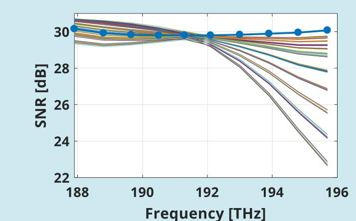
For optimal tilting we used GGN model to explore tilts between 0% and 200%. **50/0** (50% pre-compensation on L-band and 0% on C-band) is the tilt strategy which maximizes and flattens the SNR.
