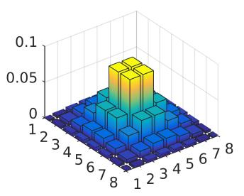
Possible solution: transmit standard QAM symbols with different probabilities!
