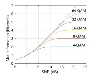
At low SNR, gap to capacity is significantly reduced
