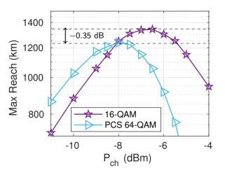
31 × 16 GBaud transmission over 80-km spans of NZDSF
