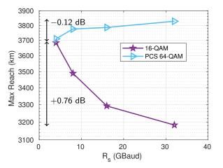
Split-step simulations of 15  $\times$  32 GBaud and 120  $\times$  4 GBaud signals over 100-km spans of SMF
